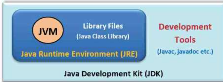
Fig: 4.3 Java Environment Structure (JDK, JRE and JVM)
