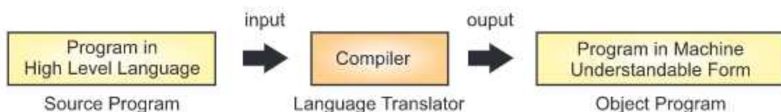
Fig. 6.6 Working of Compiler
