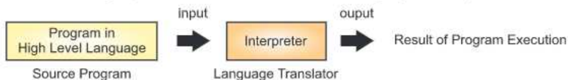
Fig. 6.5 Working of Interpreter
