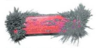
Fig 13.9 Iron filings sticking to a bar magnet.
