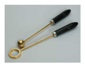
Fig. 6.6 Ball and ring apparatus
