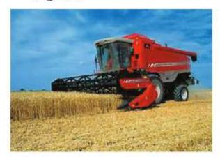
Fig. 5.6 Threshing by Machine (Combine)
